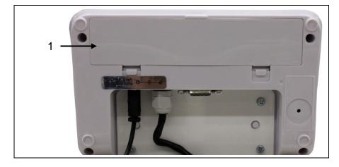
11.6 Battery operation is possible by obtaining an optional battery power pack
