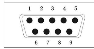
Pin 2: TXD - output Pin 3: RXD - input Pin 5: GND - signal ground
